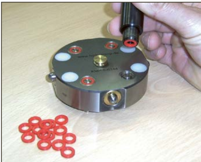
The mounting tool that is equipped with a sealing ring makes the exchange of the sealing rings easier and faster
